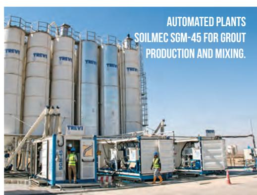
AUTOMATED PLANTS SOILMEC SGM-45 FOR GROUT PRODUCTION AND MIXING.
