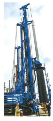
piles to depths of 19m, while the standard version offers maximum piling depths of 60m.
