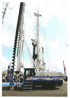
The upper structure of Soilmec's new SF-65 continuous flight auger rig is mounted on base carrier with extendable crawler frames and turret, and can rotate 360°.
