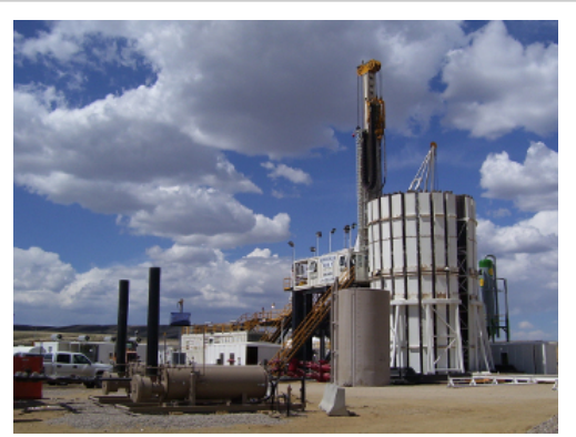
The HH Series was designed to deliver low noise, decreased environmental impact, and increased mobility for marginal field operations.
