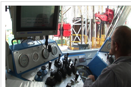
According to DrillMec, the HH Series was the first rig on the market to offer joystick controls. Today, about 80% of the routine work is done with an unmanned rig floor. (Images courtesy of DrillMec Inc.)
